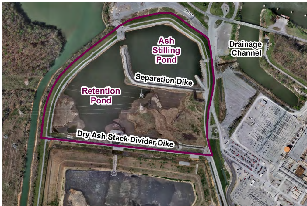
Figure 2. Stilling Pond Unit Configuration
